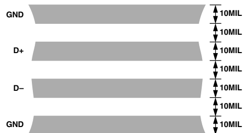
Figure 5. Arrangement of Signal Tracks
